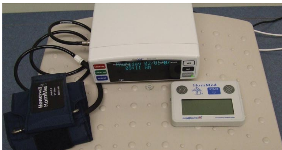
Home monitoring equipment includes a blood pressure collar, weight scale, pocket ECG and a data unit that collects and transmits information to the Heart Institute.
